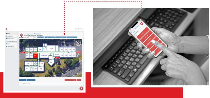
A 911 call from a cell phone automatically triggers a notification and will display the exact location on the floor plan using geofencing technology.
